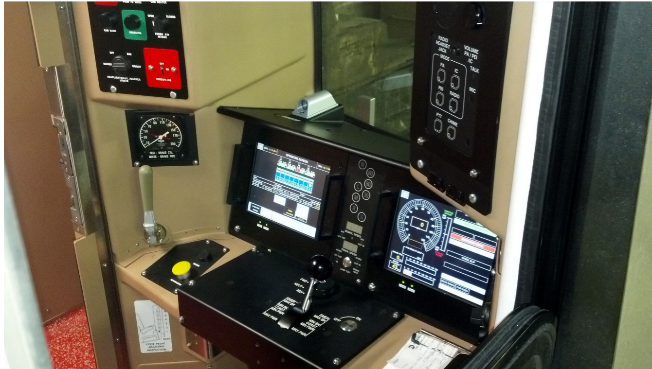
United States: Control stand in an M8 railcar operated by Metro-North.
